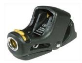
Where the rope exits the Spinlock cleat: If you pull the rope upwards whilst it is under tension, the cleat releases the rope, if you pull the rope downwards the cleat locks onto the rope. The yellow 'dial' adjusts the release spring tension and should not need adjusting.
